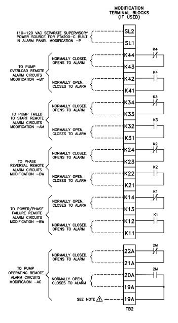
↑ SPARE TERMINALS PROVIDED FOR PARALLEL CONNECTION OF REMOTE ALARMS (IF REQUIRED)
